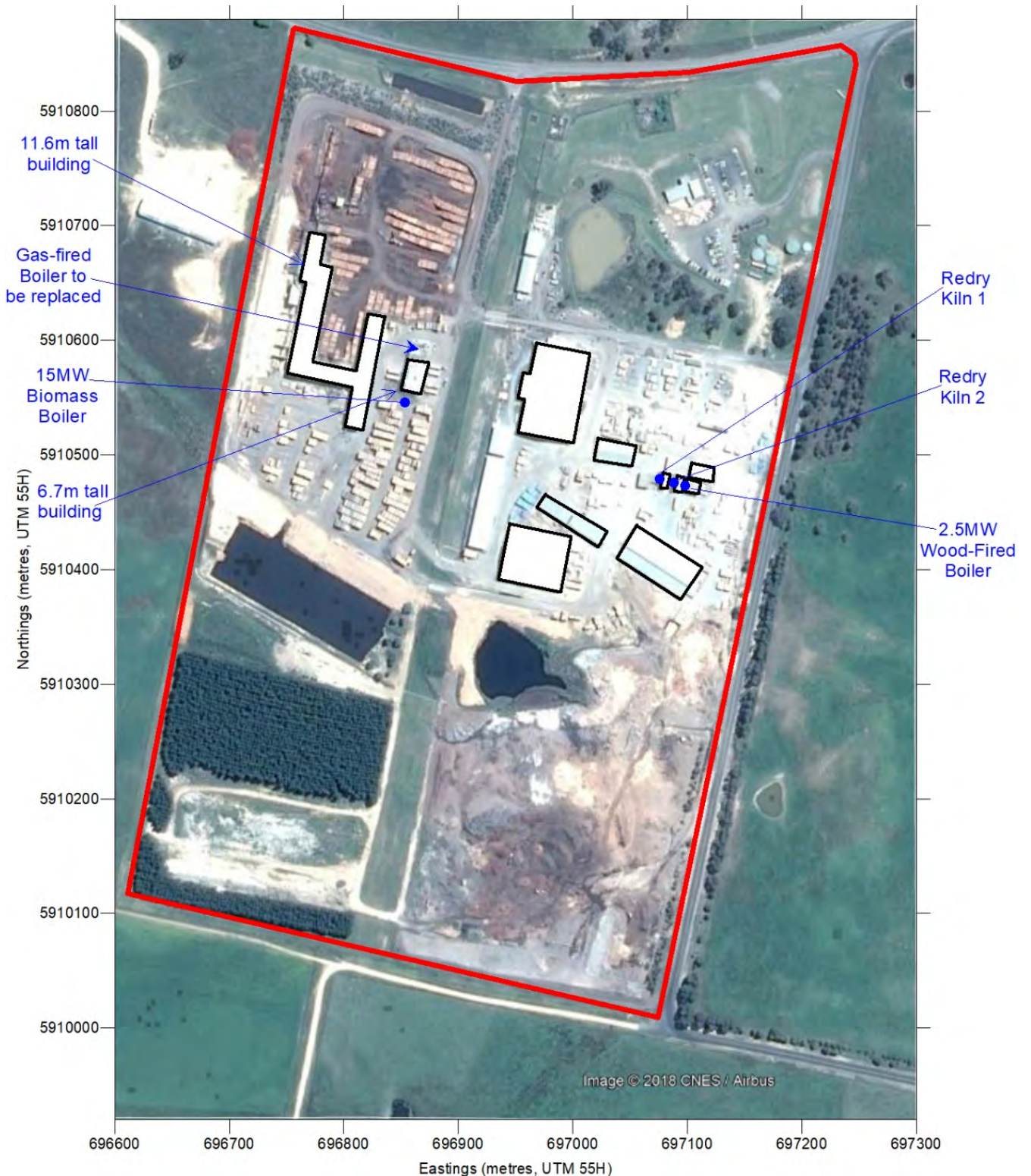
Figure 2: Extent of the DAU timber mill with emissions sources and prominent buildings indicated within the site boundary.
