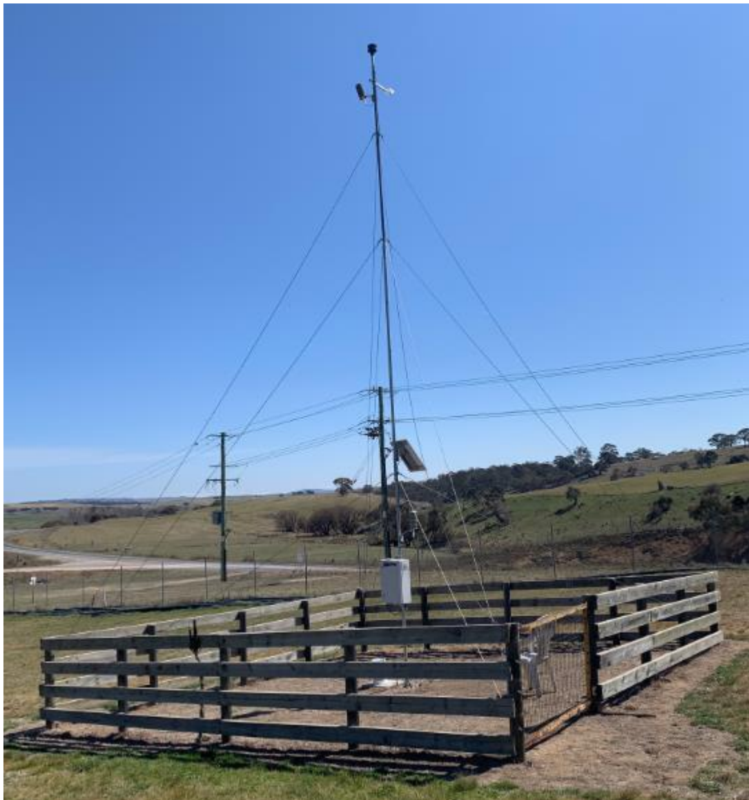
Figure 7-1: Meteorological monitoring mast
